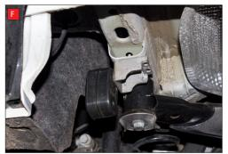
F) Both of the rear mounting points need rotating 180° when fitting the Scorpion exhaust.
